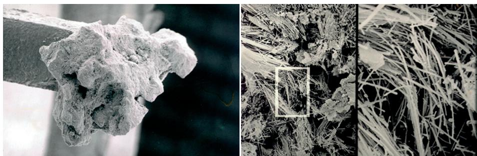
A microscopic picture of a 2 mm Aqualite™ A 100x (left) and a 1000x (right) granule enhancement.
